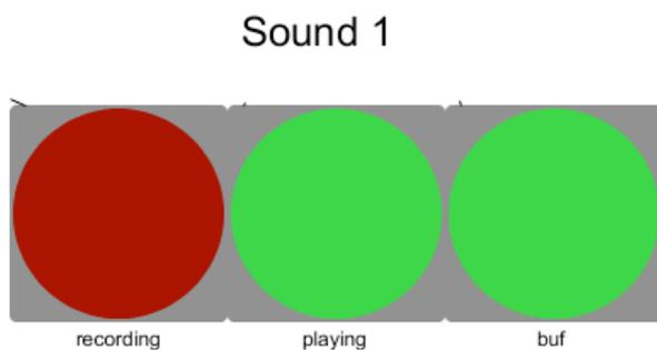
Figure 1 Three LED indicators for sound component 1, all in the off state. The first indicator highlights when recording is happening, the second when live sound is being processed, and the third when sound is played from a buffer recorded earlier.
